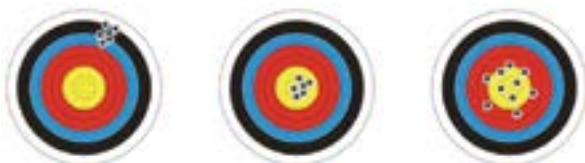
Good precision, Poor accuracy Good precision, Good accuracy Good accuracy, Poor precision
