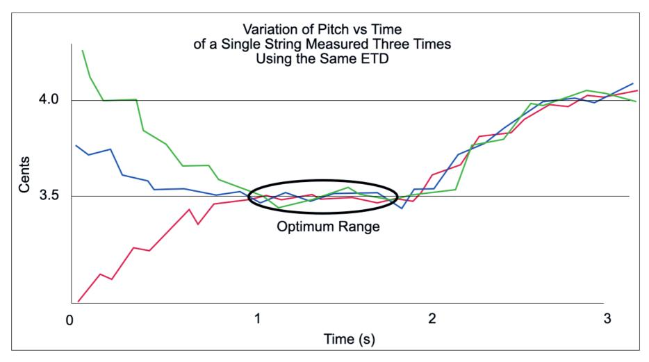
The actual time to settle can vary between different ETDs. The amount of drift and direction depends on the specific string's characteristics. This ETD was iStroboSoft which does not dampen the string's frequency like some other ETDs.
